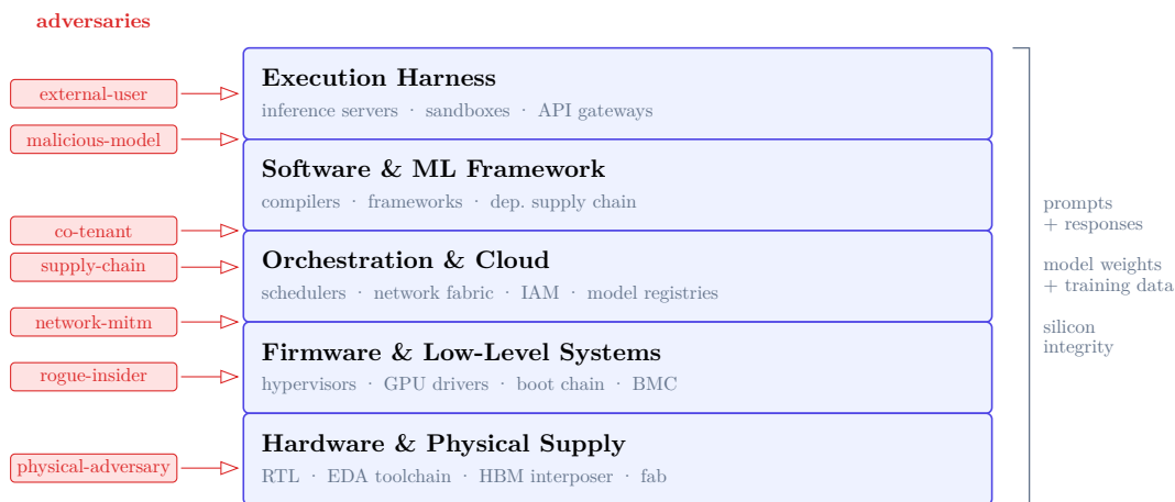
Figure 2: The five layers of the ML inference and training stack, with the adversary archetypes (left) that each layer invites and the assets (right) that pass through them. Adversaries are tagged on each layer below using the same labels; see Section 4 for full descriptions.
